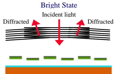
The GLV device uses digitally-generated signals to generate specific drive voltages for each pixel, achieving precise variable control over the proportion of light that is reflected or diffracted.
