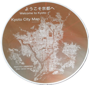
Non-Periodic High Density Write on 300mm wafer
