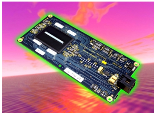
Figure 3.1: A GLV module, including drive electronics and data interface
