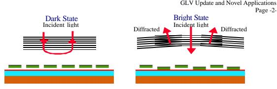
Figure 2: Reflective (dark) and diffractive (bright) states of a GLV pixel
