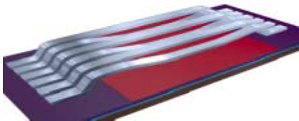
Figure 1: Typical GLV pixel, showing alternate ribbons being addressed.
